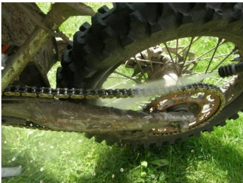
Figure 16: Motorcycle chain heavily soiled with mud is best and in the easiest way cleaned with cold pressure water without any chemicals.
