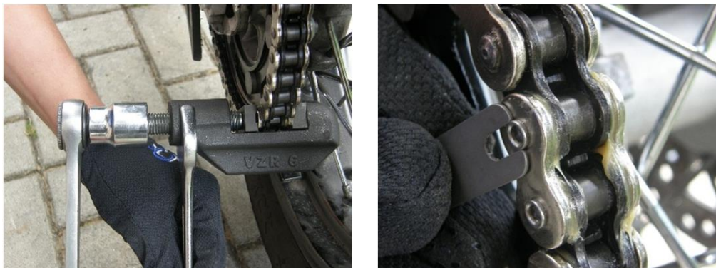
Figure 12: For proper installation of Rivet connecting links use assembly tool CZ VZR 6 and included measurement tool.
