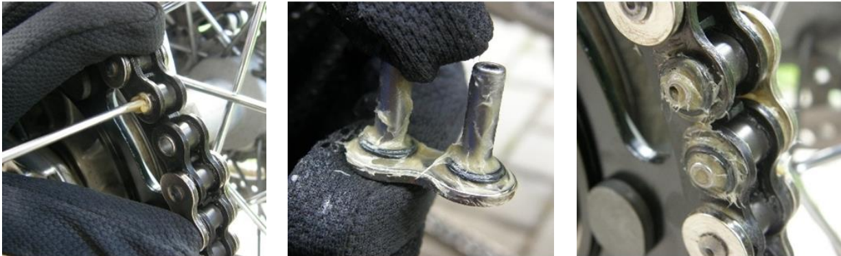
Figure 11: Proper lubrication of pins, bushes and sealing rings guarantees long term reliability of the product. With regards on perfect connection we recommend to remove unnecessary amount of lube from the connection link before riveting.
