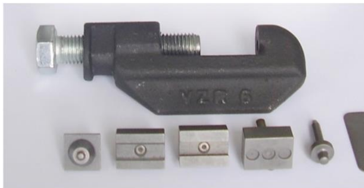
Figure 5: Original assembly/disassembly tools usable for ČZ motorcycle chains
