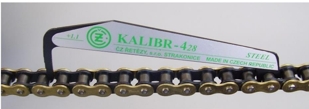
Figure 3: Checking the chain wear level by the inspection tool
