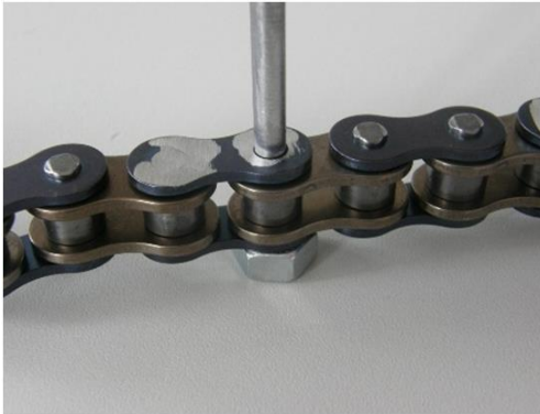
Figure 15: For alternate disconnection of the chain, see figure. For description of the procedure, see text.
