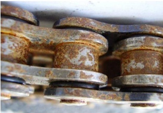
Figure 2: Rusty chain ought to be replaced as soon as possible. There is a high risk of chain destruction with possible impacts on owner's safety.
