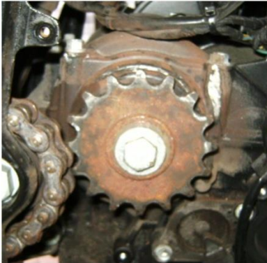
Figure 10: The chain was operated without regular lubrication, and the material seizure products of rusty colour have “powdered” on the chain wheel and engine. The chain damaged in this way had to be replaced long time ago.
