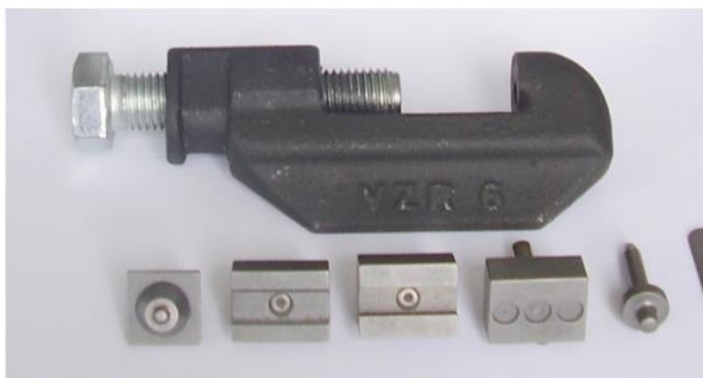
Figure 19: Assembly/Disassembly tool VZR 6
