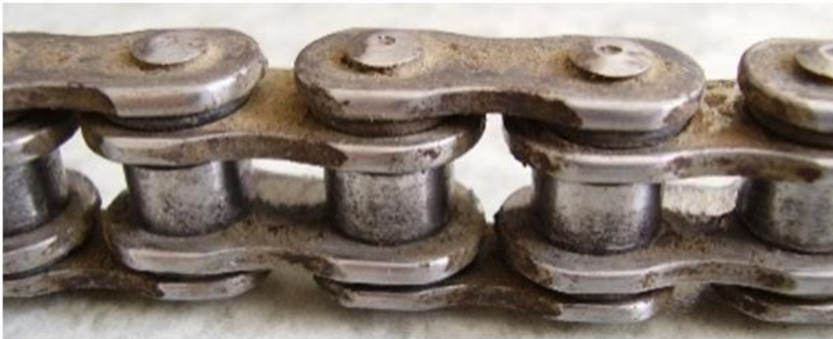
Figure 1: Excessively worn inner and outer plates
