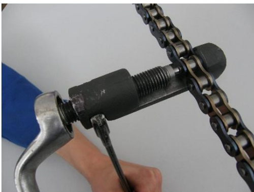
Figure 14: The VZR 6 tool is suitable for shortening of all chain types with 15.875mm pitch.
