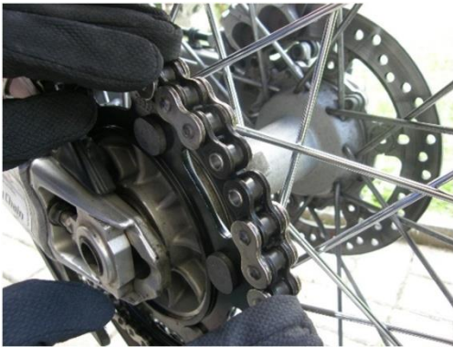
Figure 6: To measure the chain length and to assemble the connection link, it is advisable to put the chain ends on the chain wheel.
