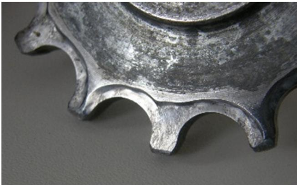
Figure 8: It is not permitted to install worn and damaged teeth of the chain wheel together with the new chain.
