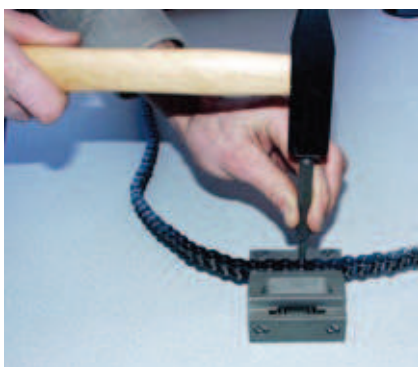
Layout13. Chain disassembly with the help of a mandrel and a hammer.
