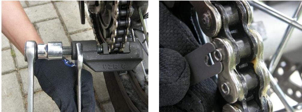
Picture 8: For proper installation of Rivet connecting links use assembly tool CZ VZR 6 and included measurement tool.
