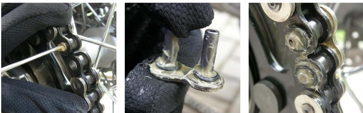
Picture 7: Proper lubrication of pins, bushes and sealing rings guarantees long term reliability of the product. With regards on perfect connection we recommend to remove unnecessary amount of lube from the connection link before riveting.
